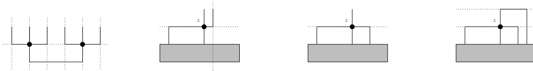
Figure 2: Embedding the first two vertices, and a singleton with in-degree 2, 3, 4. Newly added grid-lines are dotted.
